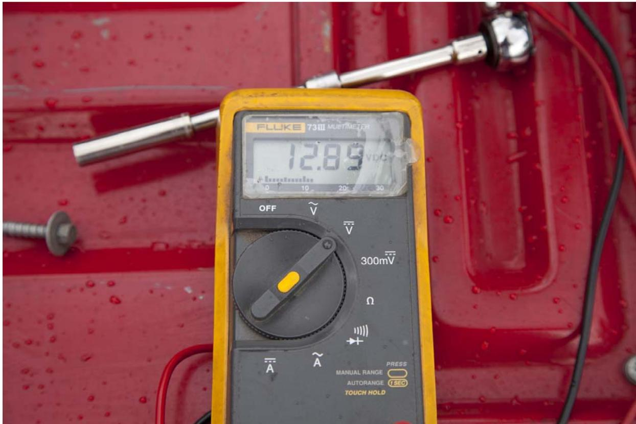
A correct reading on the voltmeter will indicate +12 volts; some voltmeters will read negative voltage, this means that you have the positive and negative wires reversed.
