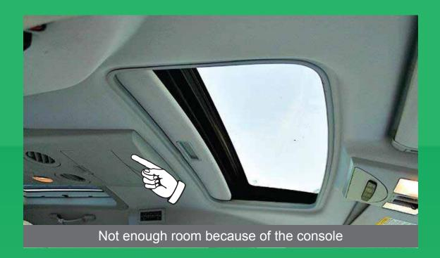
A flat surface is needed for one of our flip down units. If there is a console in the middle of your headliner, this would impede the installation of a flip down unit. A flat surface with adequate space is necessary to mount an overhead monitor. A flip down monitor will not work in this vehicle.
